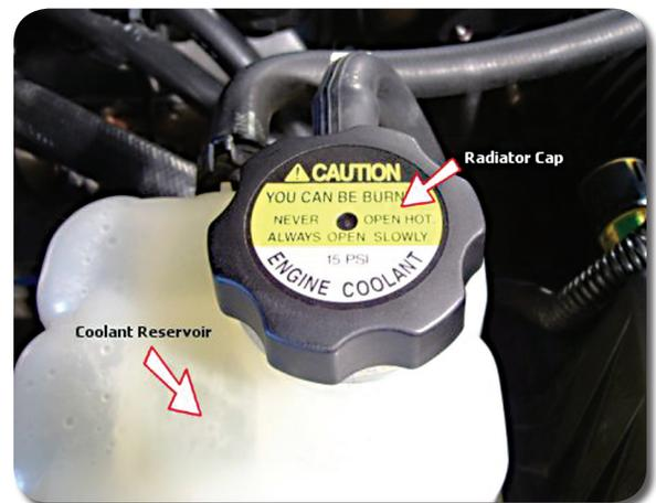
4. Unscrew the cap and add coolant to the "full" line. Coolant is a 50-50 mixture of water and antifreeze, but you can add strictly water if the reservoir's empty and your car is in danger of overheating. Adding just water is a quick and emergency measure only. As soon as possible, take your car to a professional and have them check the system out and add the proper coolant.
